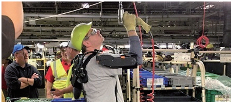
Example of improvement: A power assist device to reduce arm fatigue (North America)
